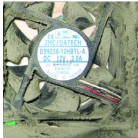
A dust covered CPU cooling fan.
